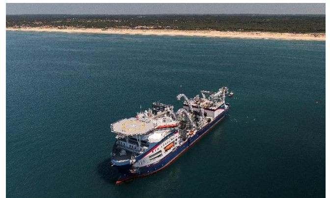
Figure 2: Cable-laying operation from the Capbreton landfall by Prysmian's Leonardo Da Vinci vessel. Credit: Llyod Images
